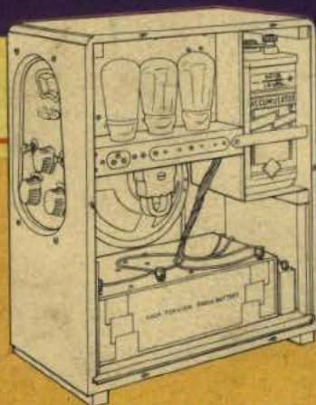
Illustration of Set with back removed, showing Standard Batteries and Accumulator in position.
