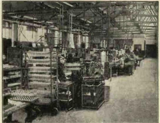
*Sealing, Exhausting and Capping Machines—
