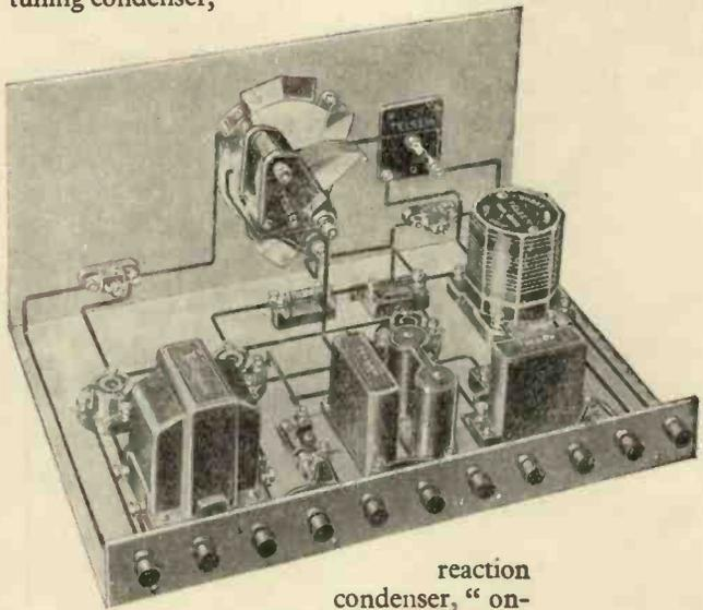
reaction condenser, "on-off" switch and wave change switch. The latter alters the tuning range from 20-40 metres (when closed) to 35-80 metres (when open). For this receiver, the valve arrangement is much the same as in the "Conqueror" Three. The output valve recommended is the P.220, as we are here concerned with maximum amplification, and we shall not expect to overload this valve. This has the
